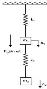
4. Apply matrix method to the system shown in the following figure and find first three natural frequencies. 14 M
